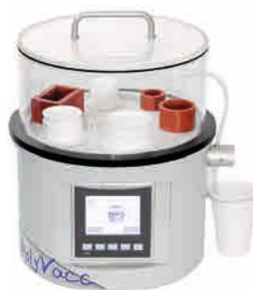
Fig 14: Vacuum mounting device: POLY'VAC
