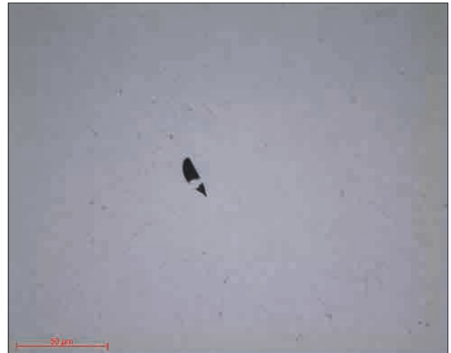
Micrograph 16: Polished stainless steel in the 1µm lens x50 state
