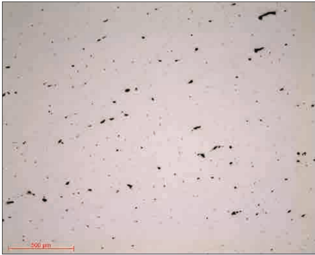
Micrograph 6: Alloy of Cobalt-Chromium - Surface condition RAM 3µm lens x5
