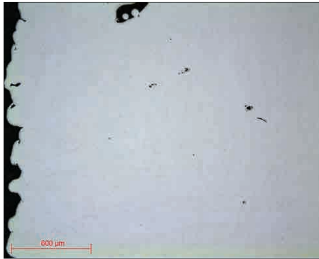
Micrograph 14: Titanium alloy - Surface condition SUPRA SPM lens x5
