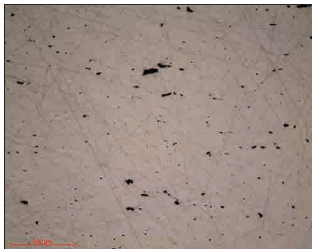
Micrograph 5: Alloy of Cobalt-Chromium - Surface condition TOP 9μm lens x5
