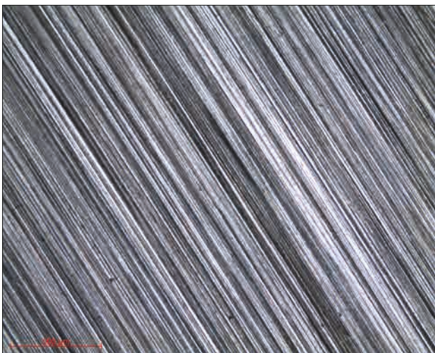
Micrograph 4: Alloy of Cobalt-Chromium - Surface condition P320 lens x5
