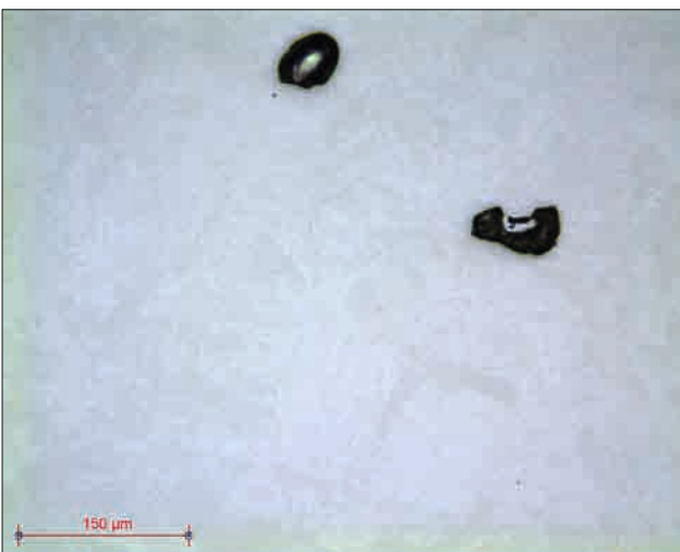
Micrographs 17 and 18: Titanium alloys polished in the SPM lens x20 and x50 state
