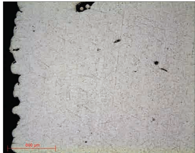
Micrograph 13: Titanium alloy - Surface condition TOP 9µm lens x5
