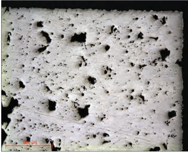
Micrograph 10: Aluminium alloy - Surface condition NT 1µm lens x5
