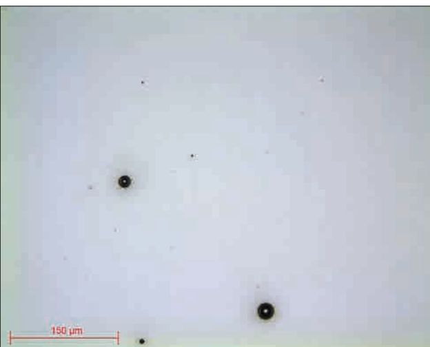
Micrograph 19: Inconel polished in Al 2 O 3 state N°3 lens x20
