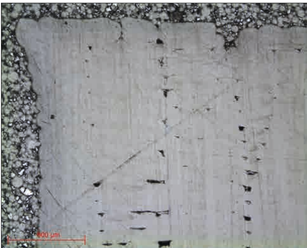
Micrograph 1: PLA – Surface condition TOP 9µm lens x5
