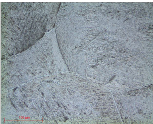
Micrograph 14: TA6V treated with Kroll lens x20 reagent etching
