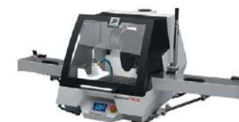
Protective tunnel for bar passage on right side - Mecatome T305/ST315 Ref. 50223
