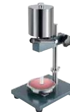
Shore hardness tester mounted on a measuring frame
