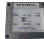
Glass roughness standards Choice of: Ra 0.8 / 1.5 / 2.2 / 2.3 / 3µm
