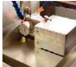
Pneumatic vice for core cutting on T265 double blade
