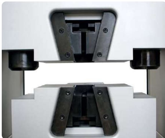
Tensile grips for flat specimens
