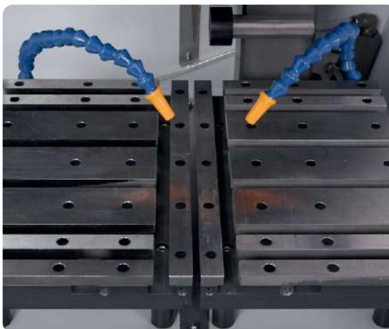
Large slotted table with stainless steel pallets
