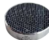
Low Load Brinell Test Block with grid
