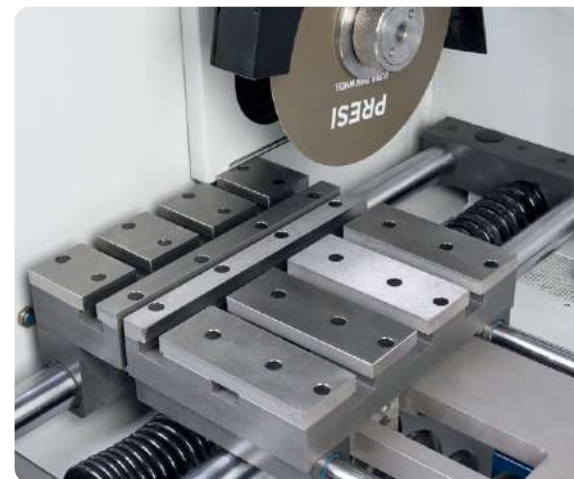
Transversal table with motorized movement Ref. 51461
