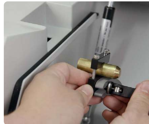
Quick clamping of sample holders
