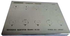
Brinell reference test block
