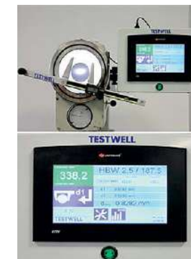
Retrofitting of hardness test machine
