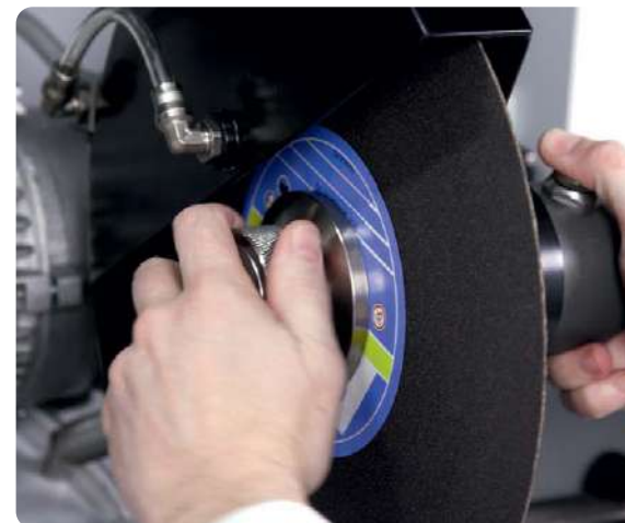
Spindle lock for wheel change with quick-release nut
