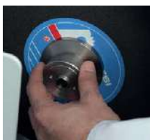
Quick-release nut for Tool-less cut-off wheel change Ref. 51272
